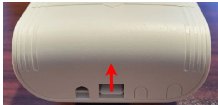
Tab that must be pulled upwards while sliding the bottom panel off.
